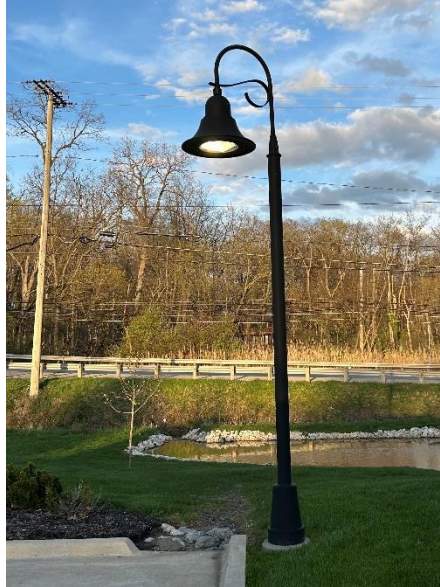
Figure 604-B – Cut-off light fixture example
